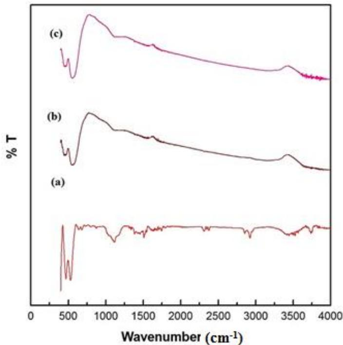
**Fig 2: FTIR spectra for a) MnFe<sub>2</sub>O<sub>4</sub> NPs, b) Co-Ni-MnFe<sub>2</sub>O<sub>4</sub> NPs, c) Co-Ni-Cd-MnFe<sub>2</sub>O<sub>4</sub> NPs**
