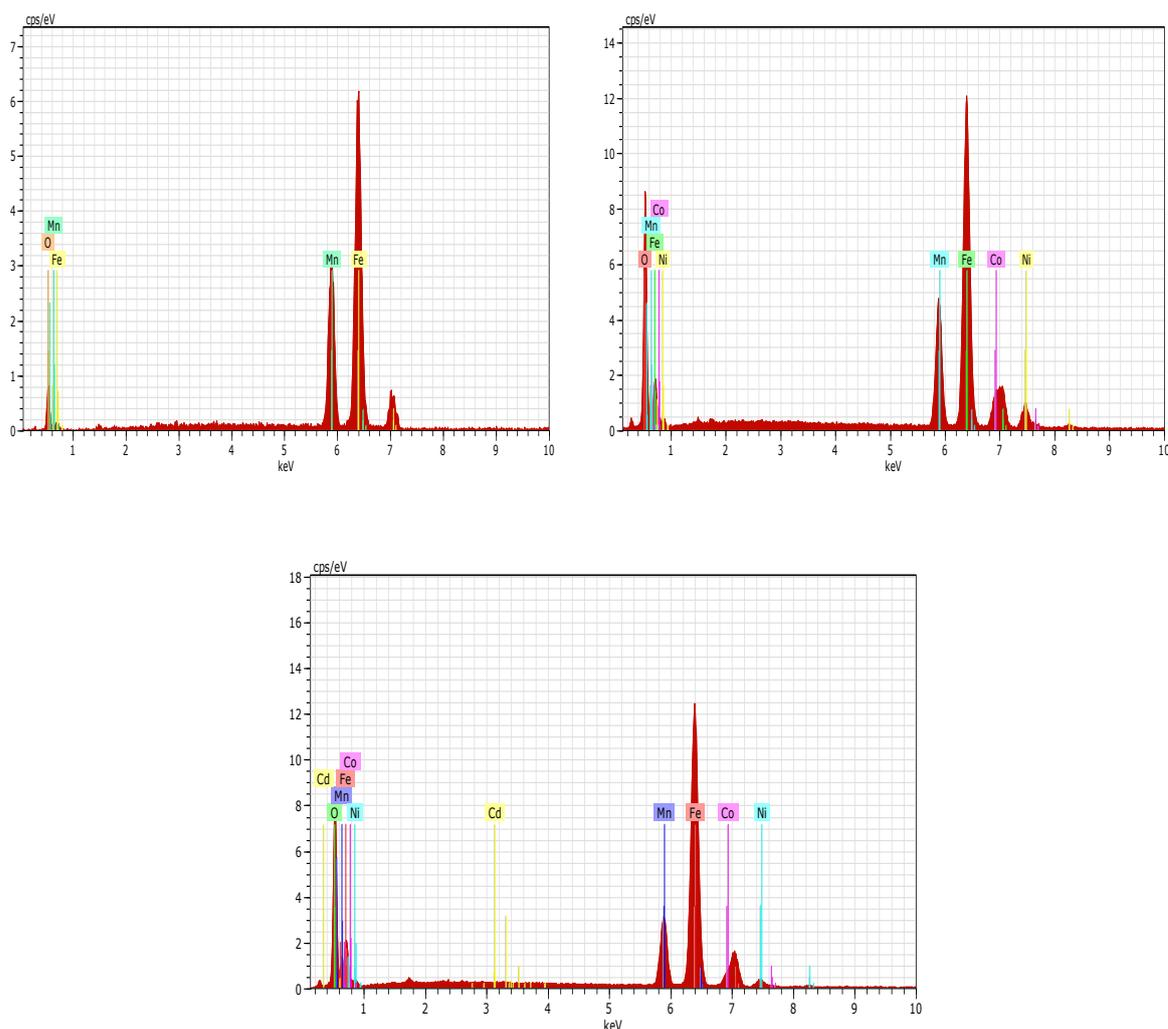
**Fig 3: EDX spectra of MnFe<sub>2</sub>O<sub>4</sub>NPs, CoNiMnFe<sub>2</sub>O<sub>4</sub>NPs and CoNiCdMnFe<sub>2</sub>O<sub>4</sub>NPs**
