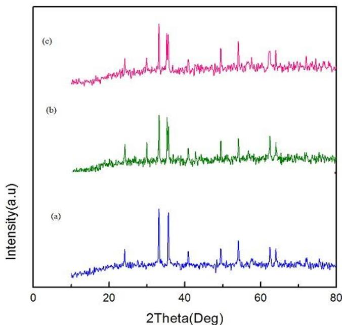
**Fig 1:** XRD patterns of the synthesized samples a) MnFe<sub>2</sub>O<sub>4</sub>NPs, b) Co-Ni-MnFe<sub>2</sub>O<sub>4</sub>NPs, c) Co-Ni-Cd-MnFe<sub>2</sub>O<sub>4</sub>NPs
